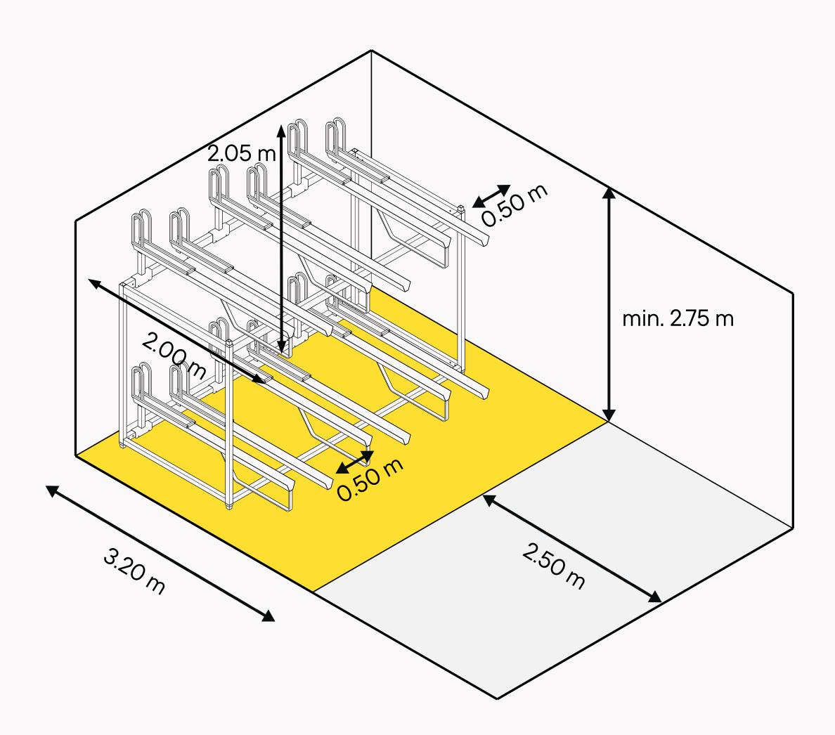
Fig. 37: Isometric drawing for bicycle parking with a double-deck parking system / © ARGUS
