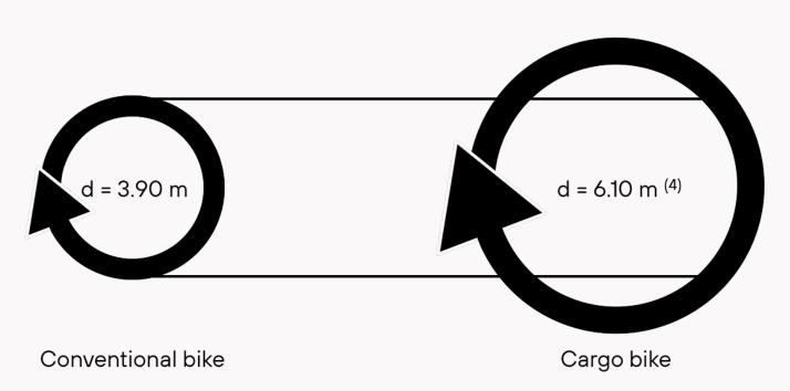
Fig. 28: Turning radii of different types of bicycles / @ ARGUS. Data based on e-lastenrad.de.
